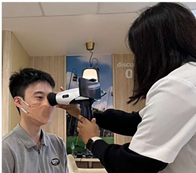
Figure 1. Demonstration of the image acquisition process using the smartphone-based oDocs Nun IR camera.
