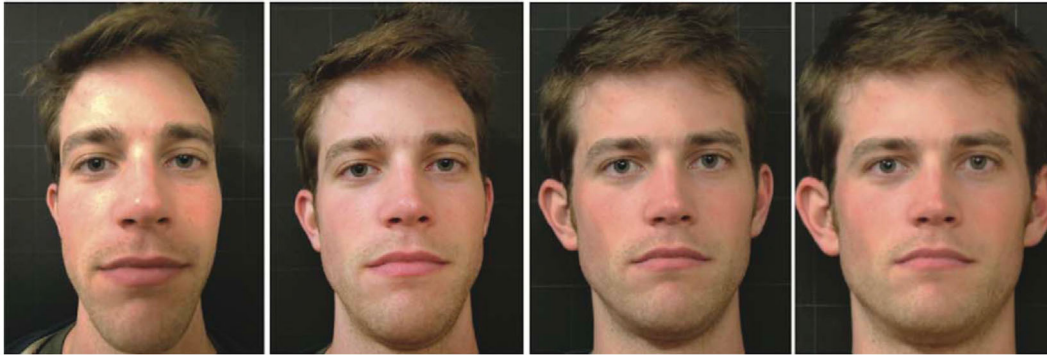
Figure 13. Facial appearance perception depends on COP distance, from Cooper et al. (2012). These four photographs of the same person were taken with four separate focal lengths: 16, 22, 45, and 216 mm (from left to right). Camera distance was kept proportional to focal length, thus keeping constant the subject's interocular distance in the picture.
